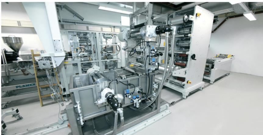
The simultaneous stretching process, which is well known as Brückner's LISIM® technology, can be analyzed in a lab scale by using the cast film of the LBE and perform the stretching in a separate step at the lab stretcher Karo IV in both directions, or in a roll-to-roll process at the pilot line LISIM® oven.
