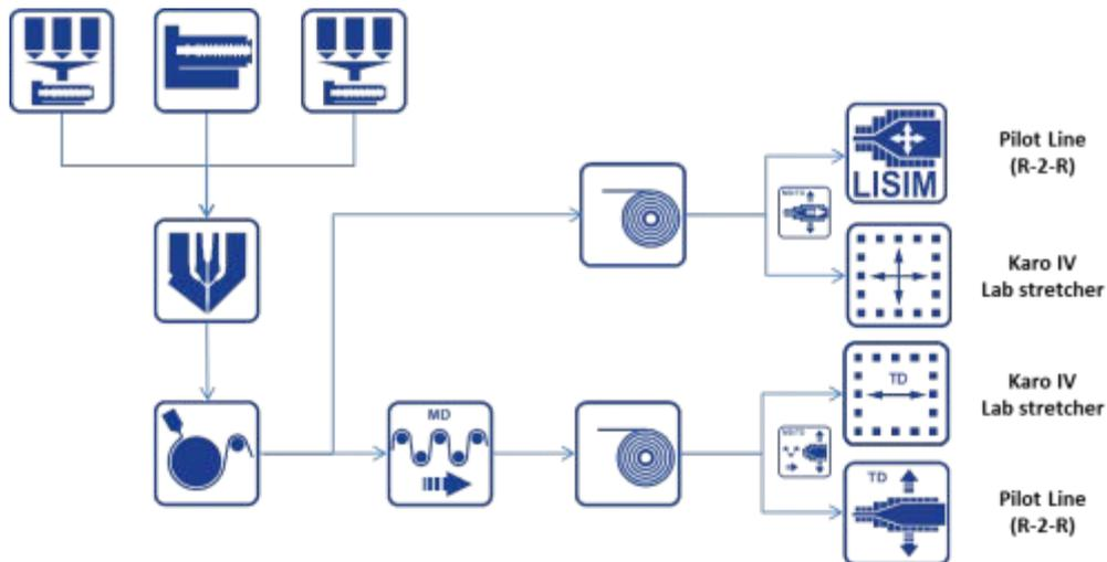
The LBE is designed to process all materials which are suitable for biaxial stretching. Also the new Evapore® process for producing PE-based battery separator film is implemented on this new laboratory extrusion line in order to test new recipes and process developments.
