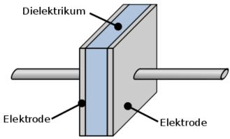
Either ceramic or plastic film is used for the dielectric. Ceramic capacitors are very small, and are used in mobile phones. Film capacitors are used in larger devices, such as in TVs and vacuum cleaners and also in electric trains and wind generators.
