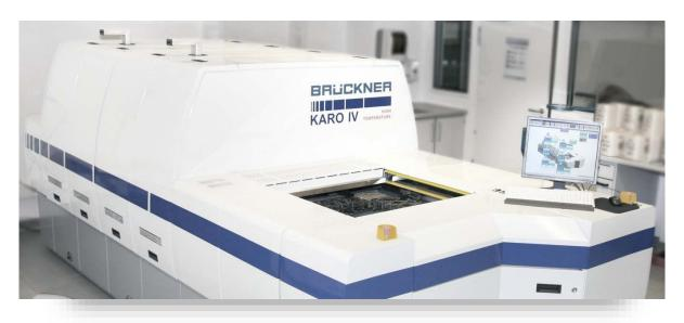
A unique facility of our technology center is our KARO IV lab stretcher. In two high temperature chambers, film samples of  $90 \times 90$  mm are heated up and stretched at temperatures up to  $400^{\circ}$ C. The lab stretcher is a compact tool for any basic analysis of stretching parameters and related film properties in a short time. This data can be implemented for pilot line or even production line operation.
