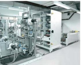
The new laboratory extruder consists mainly of one main extruder and two satellite extruders enabling the creation of up to 3-layer plastic films with optional MDO stretching. The twin screw extrusion with 56 D length gives good mixing and degassing function.
