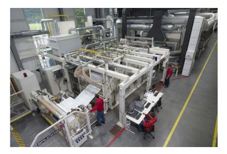
The pilot line was established in 1998 and is upgraded each year and tuned for new film types and applications. The proven LISIM® technology for simultaneous stretching as well as sequential biaxial or mono-axial stretching is used as a platform for our own developments as well as service for our customers.
