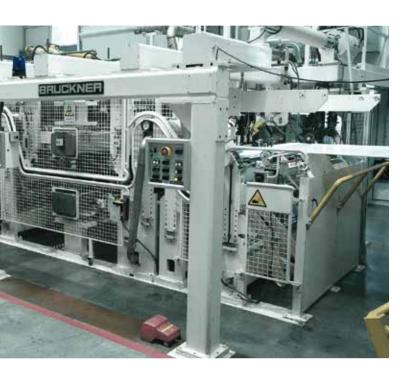
The winder allows gap and contact-winding up to a net-film width of 1.2 m. Programmable tension and contact pressure curves are used to adapt the winding characteristic to the individual film types.
