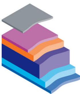
Figure 1: Typical structure of a 5-layer UHB-barrier film.
